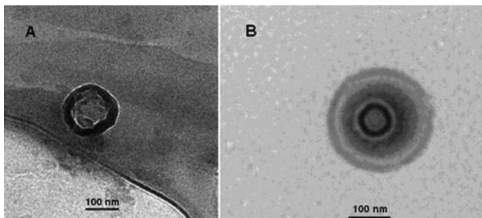
**Figure 1** TEM micropicture of PEG-*b*-PAEMA-*b*-PHFDA-1 micelle without (A) and with cross-link (B).
