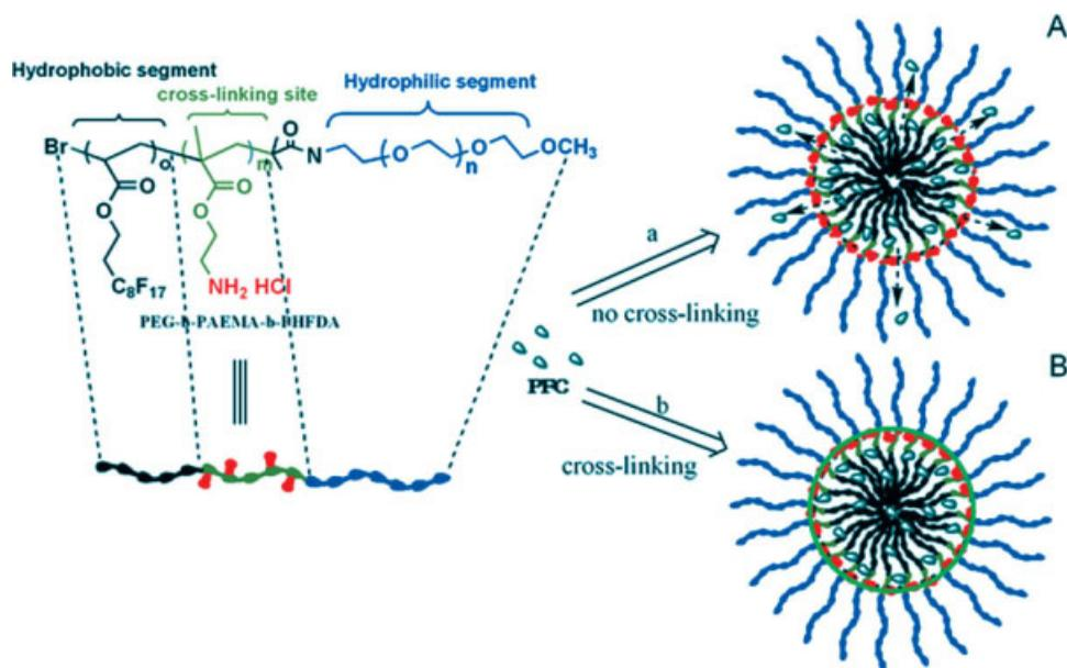
**Figure 3** Self-assembly of copolymer micelles from an amphiphilic triblock copolymer PEG-*b*-PAEMA-*b*-PHFDA for encapsulating PFC (perfluoropentane in this case) to form liquid-filled micelles using cross-link (A) or not (B). [Color figure can be viewed in the online issue, which is available at [www.interscience.wiley.com](http://www.interscience.wiley.com).]
